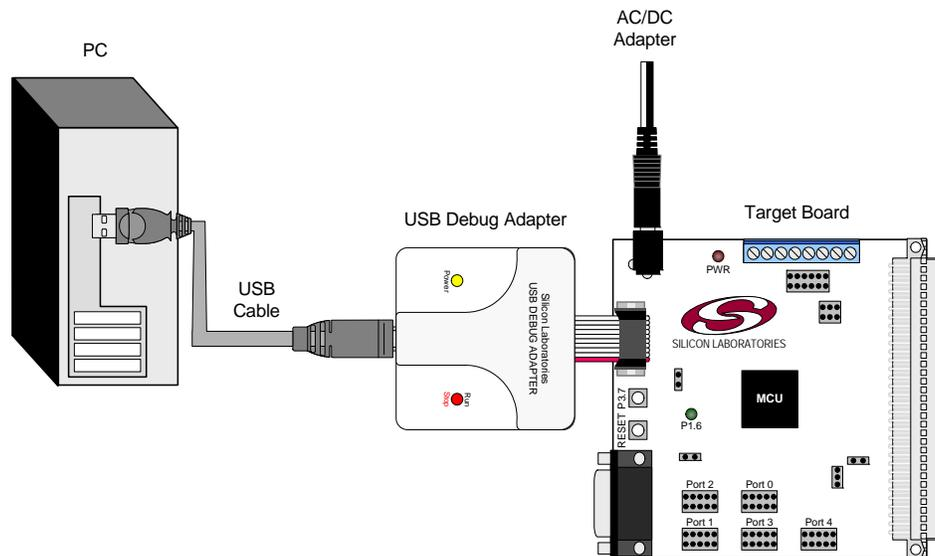
Figure 1. Hardware Setup Using a USB Debug Adapter
