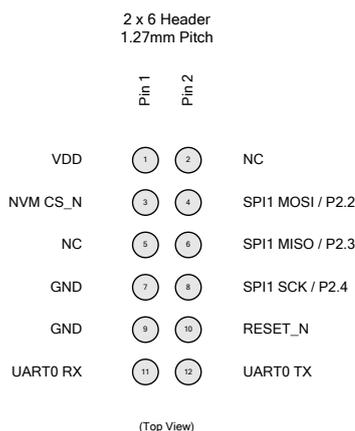
Figure 3.1: Z-Wave SPI ISP interface (SD3502, ZM5101, ZM5202)
