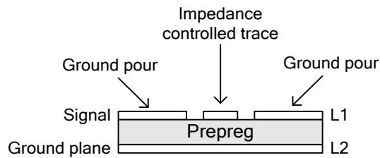
Figure 9.5: Coplanar waveguide
