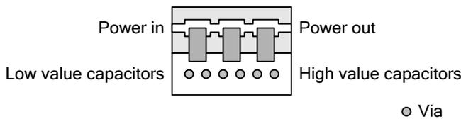
Figure 9.3: Grounded components
