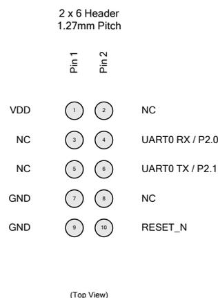
Figure 3.2: Z-Wave UART ISP interface (SD3503, ZM5304)
