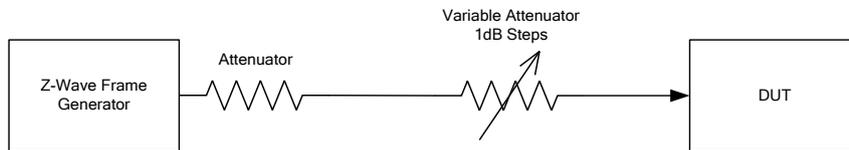
Figure 8.3: Measuring receiver sensitivity
